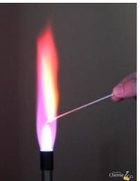
Magnesia rods are used e.g. for flame tests in qualitative analyses.
